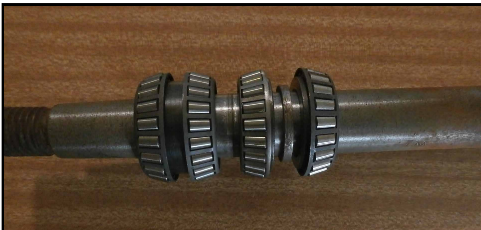
MT14 Original fit double cone on the left and the Australian Bearing Setup on the right showing spacer between two single cones.
